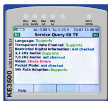
ISDN/POTS Test Telephone
